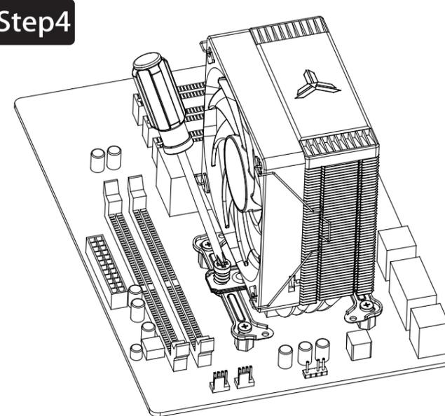
Place the cooler on the CPU while aligning the screws to the backplate mounting points, secure with screwdriver.
