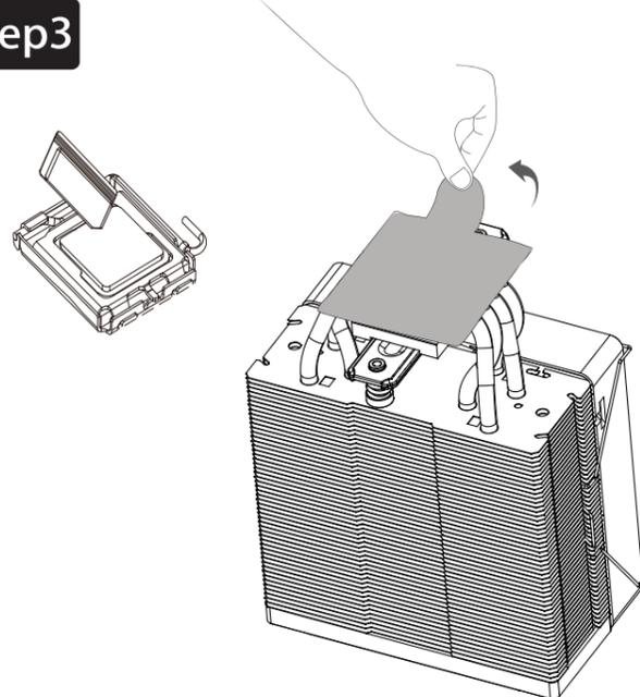
Applying the thermal paste on CPU evenly, and remove the protection film from copper base
