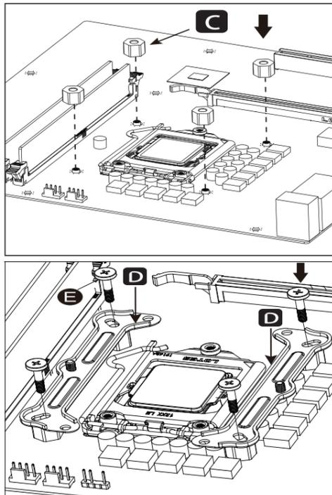
Install the mounting brackets and secure with screw
